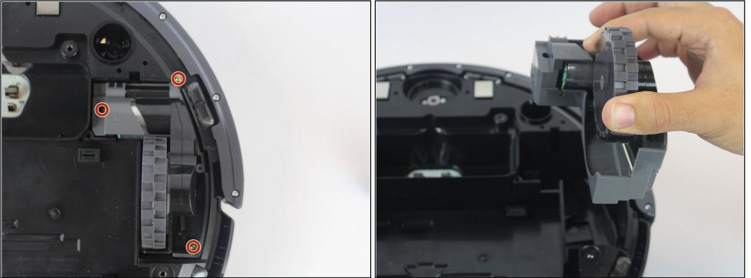
ⓘ Removing the brush module may ease the removal of the wheel module
