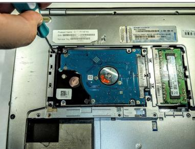
Remove the three 5mm Phillips head screws that secure the Hard Drive bay to the back panel.
