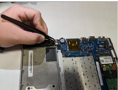
Using a pair of tweezers, remove the two cables connecting both speakers to the motherboard panel.
