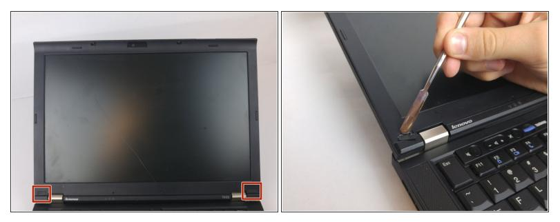
Use a spudger to remove the plastic covers from the LCD screen.
