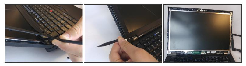
• Continue along the edges lifting up and prying off the plastic LCD bezel.
