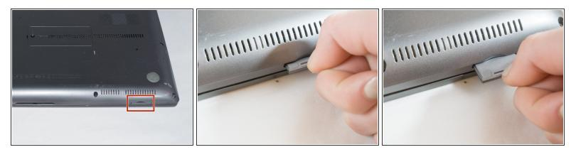
• Using your fingers, pinch the edge of the SD card and pull to remove it.
