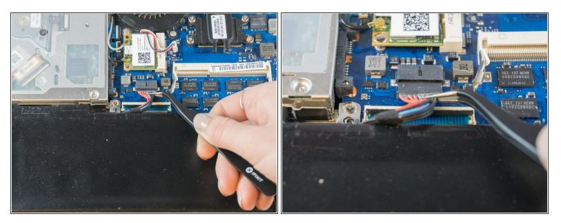
Using tweezers or your fingertips, carefully pull on the battery connector to disconnect it from the motherboard.
