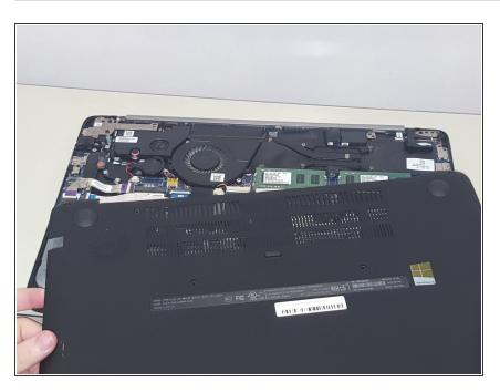
Carefully remove the back panel to reveal the inner components. To reassemble your device, follow these instructions in reverse order.
