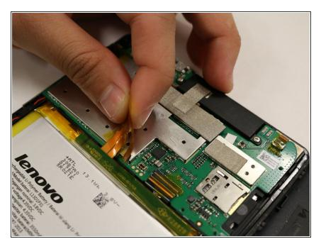
Gently detach the connector from the motherboard by pulling up on it.
