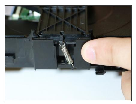
Remove spring on the side of the disc tray by carefully pulling it off its hook.
