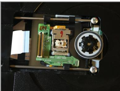
• To remove the ribbon cable, flip down the black bar located on the connector.
