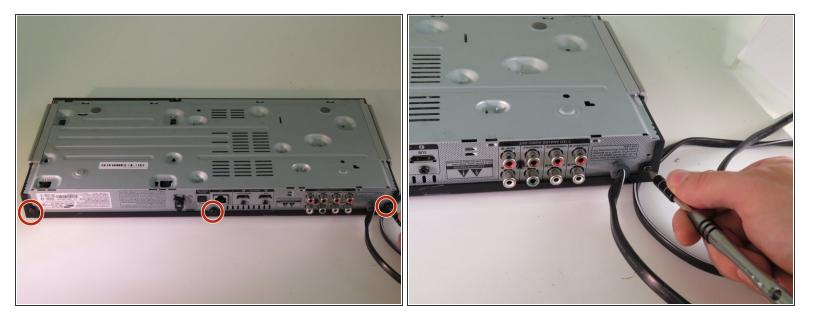
• Use a Phillips head #J1 screwdriver to remove all three (3) 10 mm screws.
