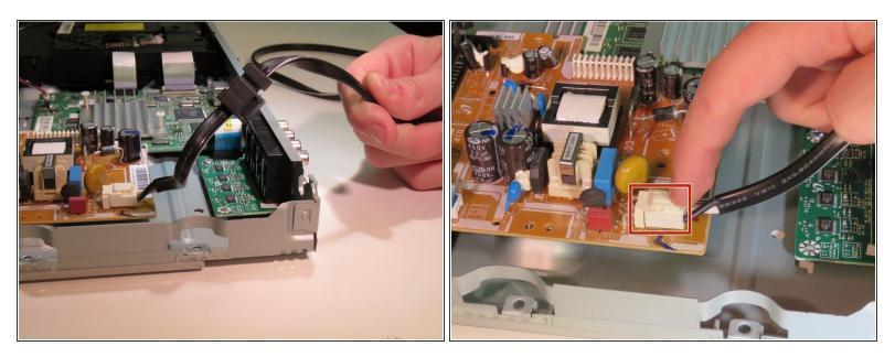
To remove the power cord, gently apply pressure to the tab located at the base of the cord and lift the cord with your fingers.
