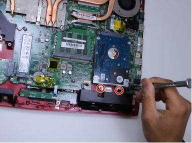
Remove the two 5.5mm screws with the Phillips #1 screwdriver.
