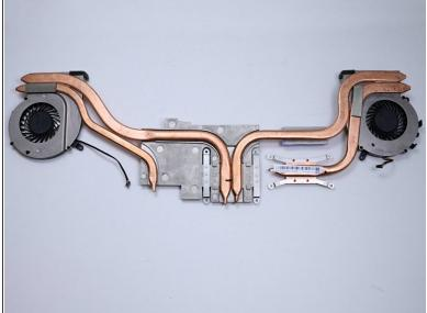
Fully remove the fans from the rest of the laptop.
