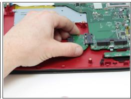
Use the Phillips #0 Screwdriver to remove the two 4mm screws that are holding the SATA connector in place.
