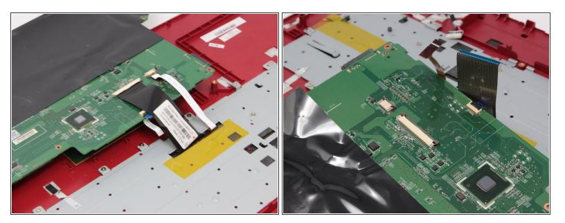
Disconnect the keyboard from the motherboard by carefully sliding the connectors out of the connections on the motherboard
