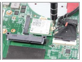
Remove the WIFI card by disconnecting the two coax cables and removing the retaining screw.
