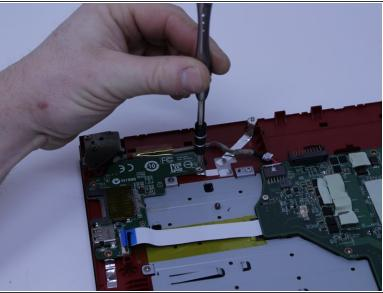
Remove the SD card reader by unscrewing the two 3 mm screws that hold it in place.
