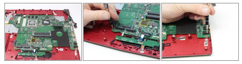
Use the Phillips #0 screwdriver to remove the three 3.8 mm standoff screws that retain the motherboard and carefully remove it.
