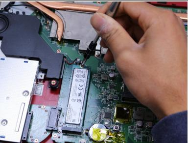
Remove the single 5.5mm Phillips #1 screw attaching the SSD to the laptop.
