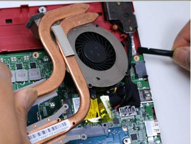
Continue to use the spudger to carefully separate the wires of the power cord from the laptop.
