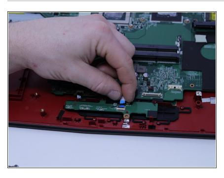
Disconnect the motherboard from the mouse key control board by pulling the connector out.
