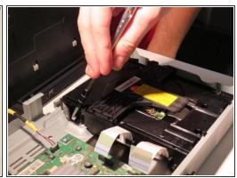
Using a screwdriver with a #J1 bit, remove the two (2) 7 mm screws.
