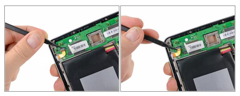
Use the tip of a spudger to carefully flip up the retaining flap on the power and volume button ribbon cable ZIF socket.
