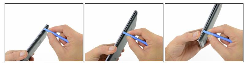
Insert the plastic opening tool between the rear panel and the front panel assembly near the power button and pry up at several points along the right edge of the Nexus 7.
