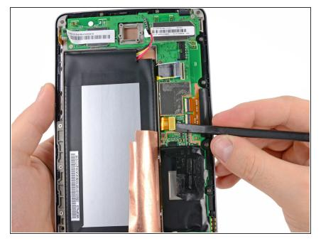
Use the flat end of a spudger to pry the display data cable straight up off its socket on the motherboard.
