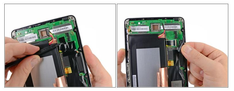
Carefully peel back the adhesive tape covering the I/O board ribbon cable socket on the motherboard.
