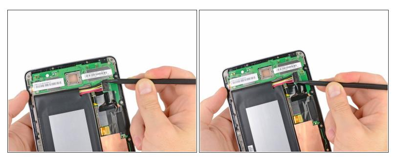
Using the tip of a spudger, push first on one side then the other to "walk" the battery cable straight out of its socket on the motherboard.
