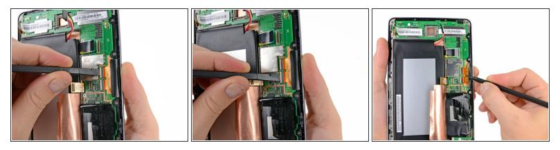
Use the flat end of a spudger to carefully flip up the retaining flaps on the digitizer ribbon cable ZIF sockets.
