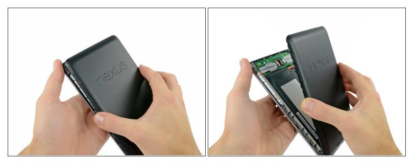
• Gently lift and remove the rear panel up off the front panel assembly.
