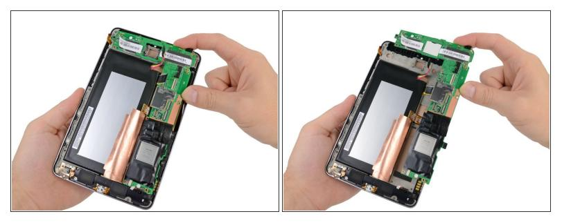
Carefully lift the motherboard assembly out of the Nexus 7, minding any cables that may get caught.
