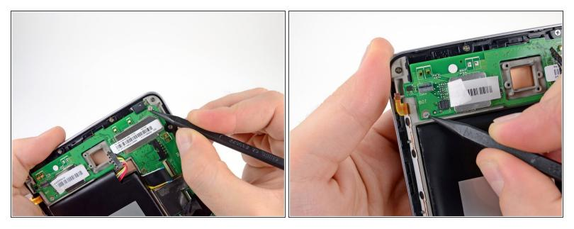
• Use the tip of a spudger to remove the warranty seal stickers.
