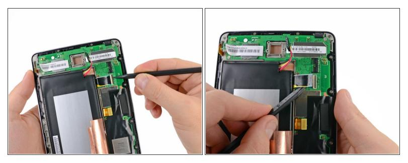
Use the tip of a spudger to carefully flip up the retaining flap on the I/O data ribbon cable ZIF socket.
