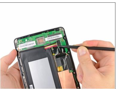
Using the tip of a spudger, push first on one side then the other to "walk" the battery cable straight out of its socket on the motherboard.
