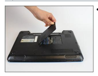
Once the RAM cover is free use your hand to pull from the side with the screw: UP and OUT to remove the RAM cover.
