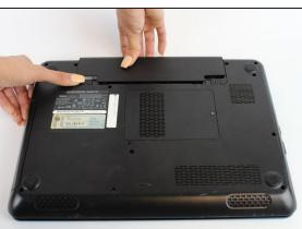
• While holding the left-hand switch to the left position, pull the battery away from the laptop.
