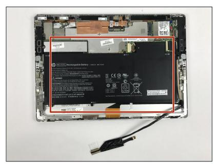
The battery for this device is under the screen and takes up most of the space.
