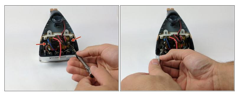
Use the Philips head #0 screwdriver to remove the two 9.75mm screws (left and right) affixed to the circuit board.
