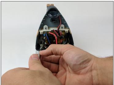
Use the Philips head #0 screwdriver to remove two 9.75mm screws (left and right) affixed to circuit board.
