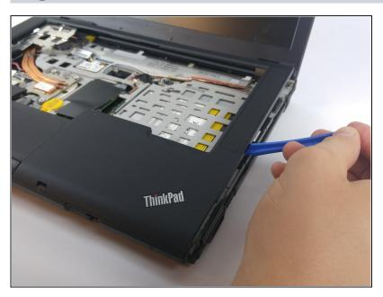
Snap off the top cover with a plastic opening tool, ensuring that the tabs don't snap back on.
