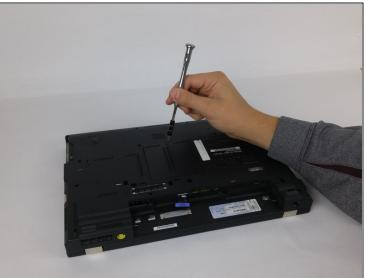
• Loosen (do not remove) the 14.0mm screw in the DIMM slot cover with a Phillips #2 screwdriver.
