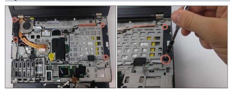
• Remove the four 3.0mm screws with a Phillips #0 screwdriver.
