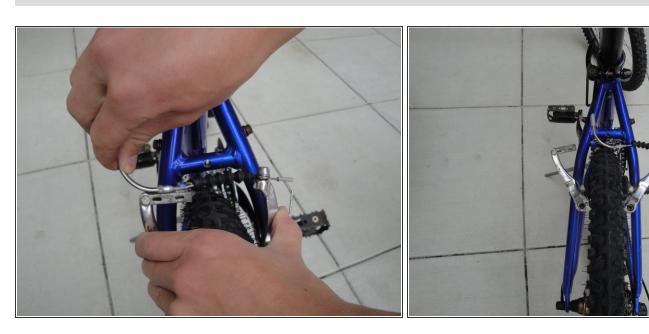
Reattach the brake cable to the calipers
