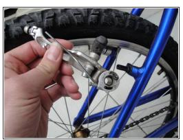
Loosen the break caliper bolt, and remove the brake caliper.
