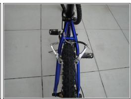
Squeeze the calipers together, and remove the brake cable.
