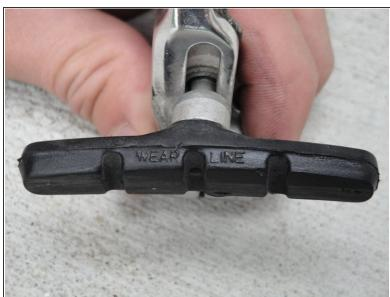
• Inspect the brake pad. If the pad has worn down past the "wear line", then it needs to be replaced.
