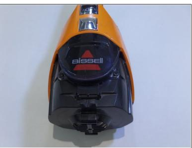
Push the silver button to disconnect the dirt dish from the handheld vacuum.
