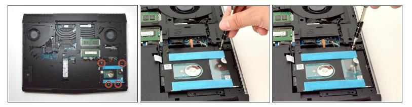
• Use a PH1 screwdriver bit to remove the four M2.5x5 screws (2.4 mm) on the hard disk drive.
