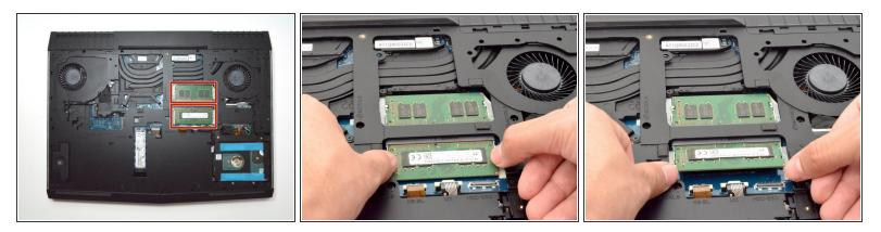
Move the metal sidings outward to release the RAM card.
