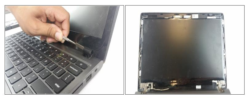
Remove the faceplate's bottom hinges that connect to the body of the device with the metal spudger. This will free the plastic perimeter, which may now be removed.
