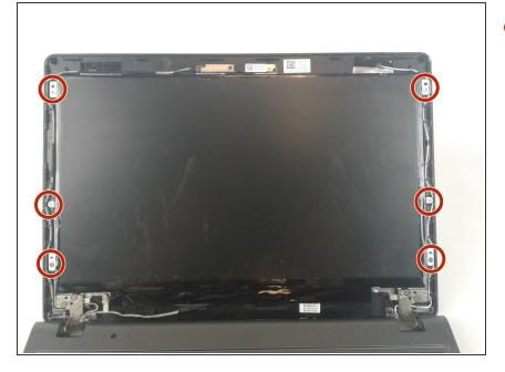
Use a Phillips #0 screwdriver to remove the 6 screws in these circled locations.
