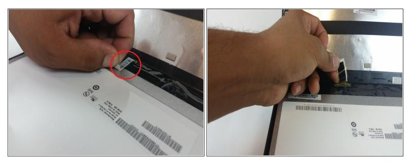
Locate the bar code adhesion strip at the base of the screen, and then peel it back carefully. Once peeled back the plug-in will come free.
