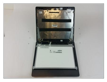
• Reposition so the screen will lay flat on the keyboard of the laptop.
