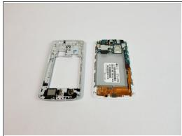
Use the plastic opening tool to remove the back housing from the frame of the phone.
