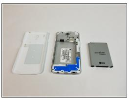
With your finger, pry the battery out through the crease made for removal.
