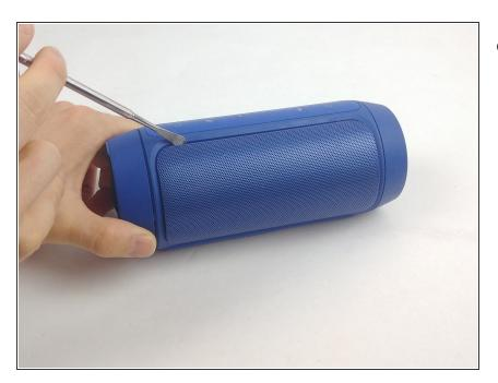
Remove the screen cover from the speaker using a metal spudger.
