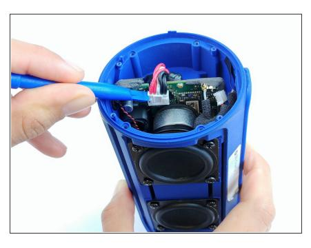
Disconnect the battery connector with a plastic opening tool and wiggle the connector free.
