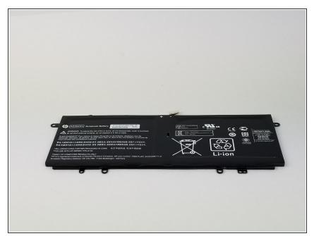
Carefully lift the battery and remove it from the device.
