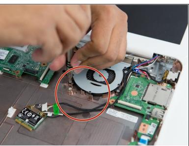
Use the Phillips #1 screwdriver to remove the (5) five screws.
