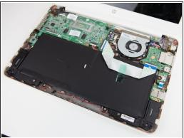
Once the ribbons are detached, remove the keyboard from the device.
