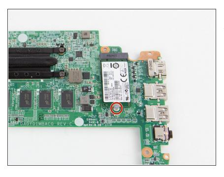
Locate the retaining screw for the SSD.
