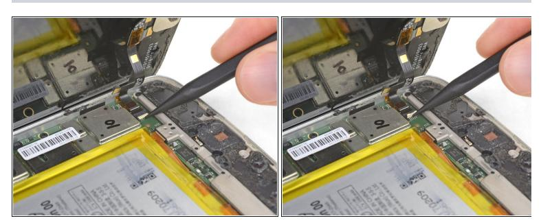
While holding the display open, use the point of a spudger to pry up the locking tab on the fingerprint sensor cable's <u>ZIF connector</u>.
