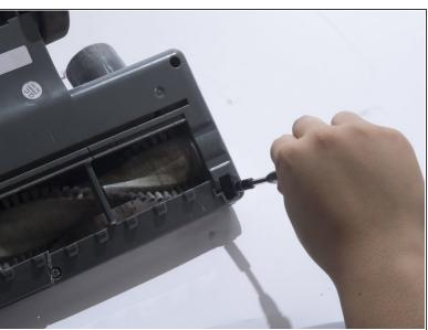
Remove the two 18mm screws with a JIS 1 screwdriver.
