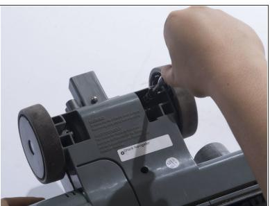
Remove the two 18mm screws located on the inside of the large wheels using a JIS 1 screwdriver.
