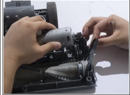
• Remove the belt from the motor gear by sliding the belt to the right.
