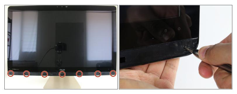
• Use a Phillips #1 screwdriver to remove the seven (7) 4.8 mm screws from the base of the screen.
