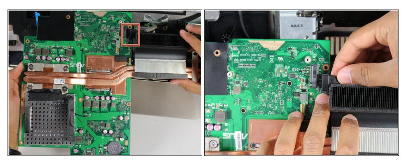
Remove the SATA cable on the opposite side of the motherboard by pulling directly up from the board.
