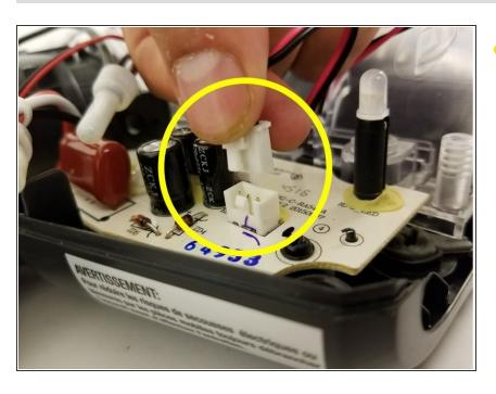
Unclip the 2-pin electrical connector
