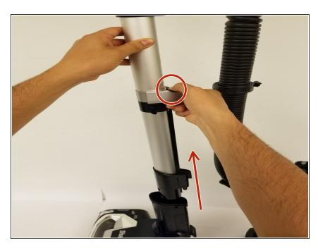
Push lift away button on the wand then lift up on the top section to separate.
