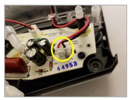
Follow the headlight's red and black wires to the circuit board.
