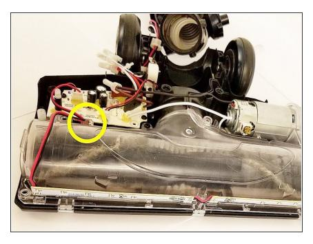
Detach the headlight's red and black wires from plastic clip as shown.
