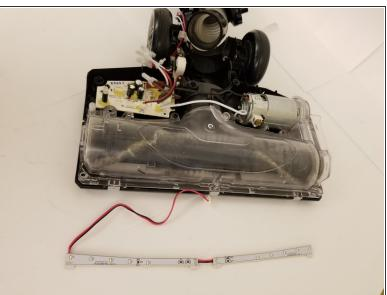
Carefully lift the headlights and its wires from the vacuum assembly.
