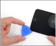
• Continue separating the glue underneath the rest of the lower bezel.
