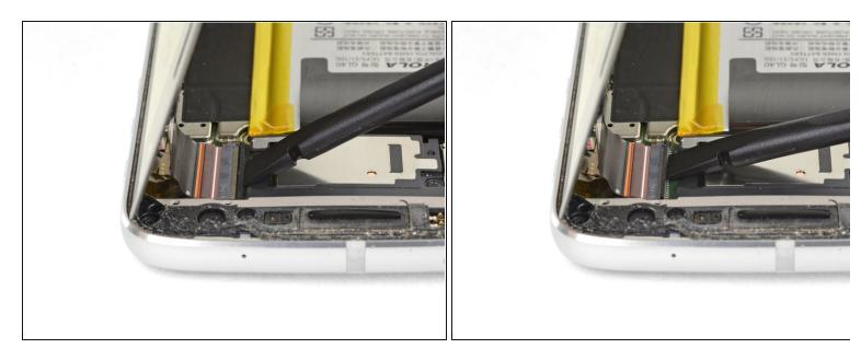
• At the opposite end of the phone, use your spudger to flip open the locking tab on the display cable connector.
