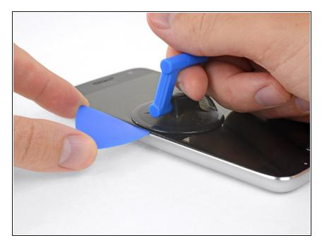
Insert an opening pick (or playing card) into the gap you opened behind the display.
