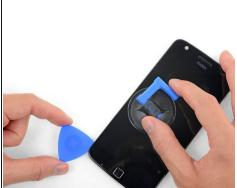
Slide the tool all along the left edge of the phone to slice through the adhesive securing the display.
