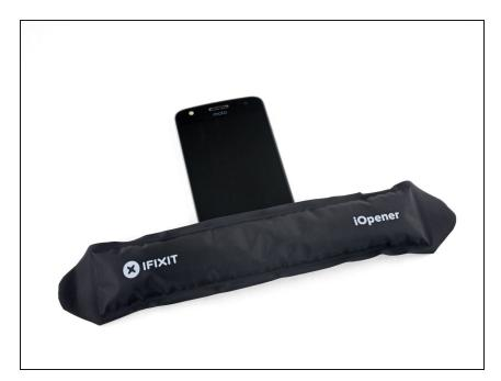
Heat the front of the phone between the display and the lower edge to soften the adhesive underneath.
