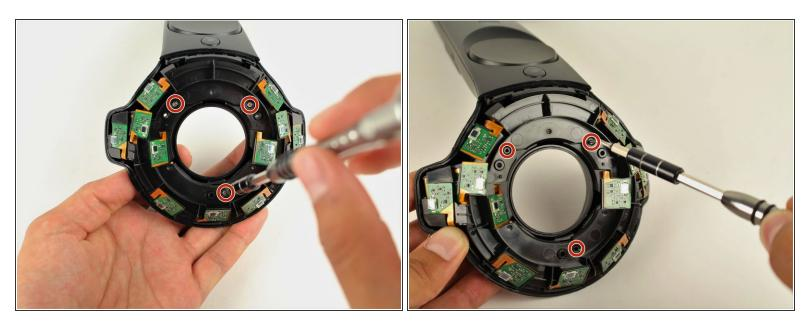
Use the Phillips 00 screwdriver to remove the three silver 12.8mm screws from the exposed upper sensor panel.
