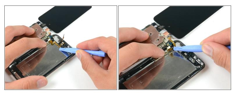
• Slide the plastic opening tool under the length of the ribbon cable to release it from the rear panel.
