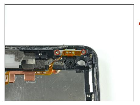
Remove the two 2.0 mm Phillips screws securing the power button assembly to the rear panel assembly.
