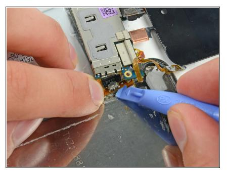
Wedge the plastic opening tool under each volume controller and pry the assembly loose from the case.
