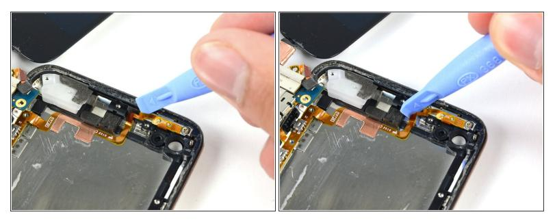
With the corner of a plastic opening tool, gently move the ribbon cable out of the way so you can get to the screw beneath it.
