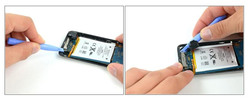
• With a plastic opening tool, carefully push the dock connector out of its outer case recess. Work each corner evenly until the connector comes free.
