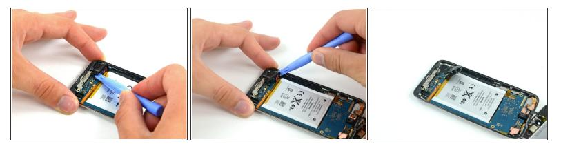
• With a plastic opening tool, gently pry the iPod's speaker out of its recess in the outer case.
