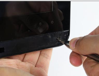
Use a Phillips #1 screwdriver to remove the seven (7) 4.8 mm screws from the base of the screen.
