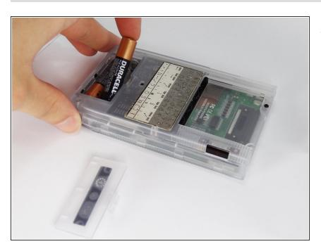
Remove the batteries from the device.
