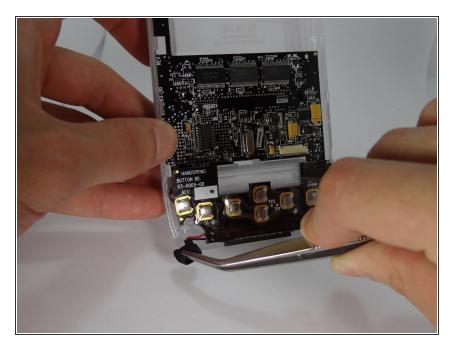
Use tweezers to remove the power button from the back case.
