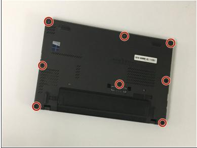
Remove the back cover by unscrewing the 8 0.2 mm screws holding it in place.
