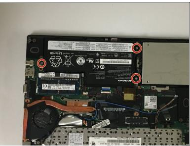
Locate the internal battery pack and unscrew the 3 0.2 mm screws holding it in place.
