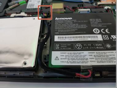
Unplug the connector cable that connects the internal battery pack to the laptop.
