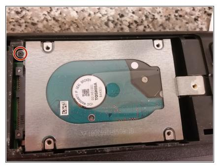
• Remove the single screw securing the hard drive caddy to the base.
