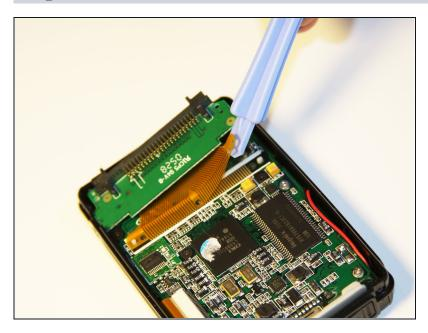
• Using the plastic opening tool, completely lift the ribbon off of the motherboard.
