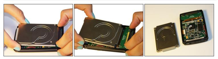
• Place fingers on the IDE connectors gently picking up and sliding the hard drive out from the IDE module.
