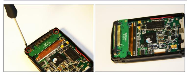
• Using the Phillips #00 screwdriver, unscrew the two 1.5mm long screws holding the IDE connector to the motherboard located at the top.
