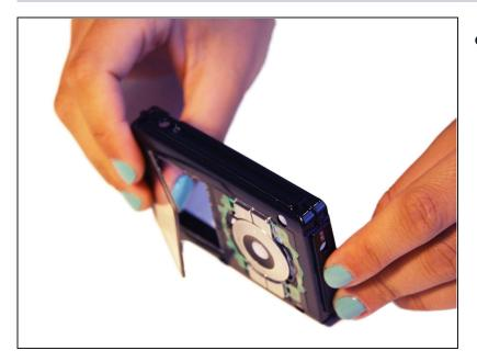
• Grasping the sides of the cover, gently press on screen protector from the inside of the front cover to pop out the screen protector.
