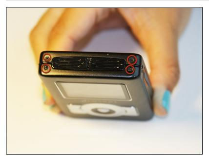
Use a Phillips #00 screwdriver to unscrew the four 1.1mm long screws on each corner located at the top of the cover.
