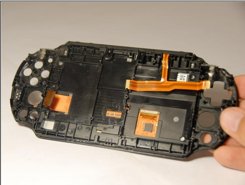
ⓘ The best way to replace the display is to replace the entire front.
