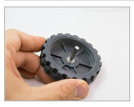
• Much better! As you can see the only thing that keeps the wheel in place is the main gear. there is no problem of the gear slipping because the axle is splined. If you want you can use some threadlock to help securing the gear. To reassemble your device, follow these instructions in reverse order.
