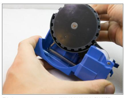
Remove the shock spring to keep the wheel from jumping off when you remove the bolts
