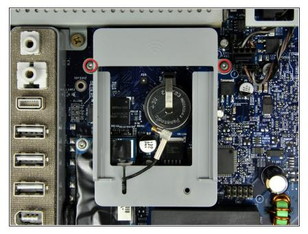
Remove the two 5.5 mm T6 Torx screws securing the AirPort bracket to the logic board.
