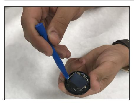
Use a pair of nylon spudgers to assist the removal of the motherboard. Pry up on two tabs and the mother board will pop out.
