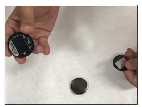
Remove polymer cover that is protecting the mother board, it should just come out when two halves are separated.
