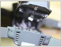
Gently lift up the rear of the top case .5-1mm, and insert a pair of tweezers, grab the black cloth shielded cable connecting the top and bottom, and gently pull it up and away from the bottom board. The rear should lift freely up from the case 2-3mm.
