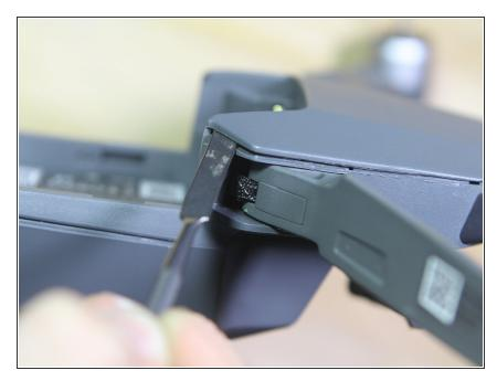
• Insert your metal spudger in between the top and bottom case on both the left and right sides of the drone, as shown in the photo. Pry up gently until it is free.
