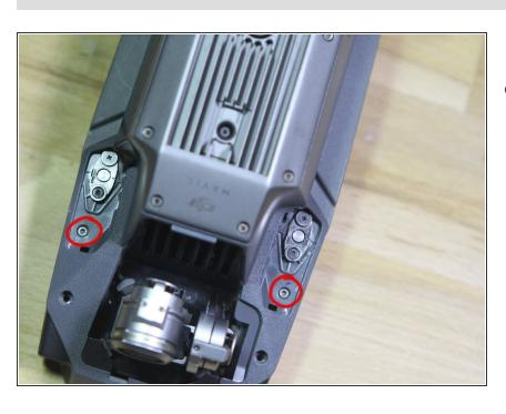
There are two 1.5mm hex screws, these are 5.8mm long, with a 2mm diameter. These are thicker than the screws holding the covers down, because those screws are only holding the covers down, while the screws under it are holding the top cover down. Take note of this during reassembly.
