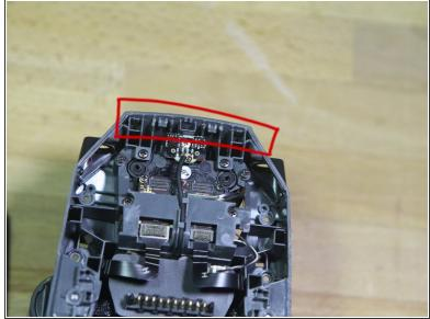
• This part is tricky. There are four clips folding the front edge in place. Half are facing one direction and half are facing he opposite direction. Be gentle and careful when disengaging them. The photos here, show the locations and directions of the clips.
