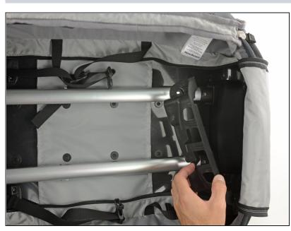
Remove the black plastic retaining bracket from the top of the frame.
