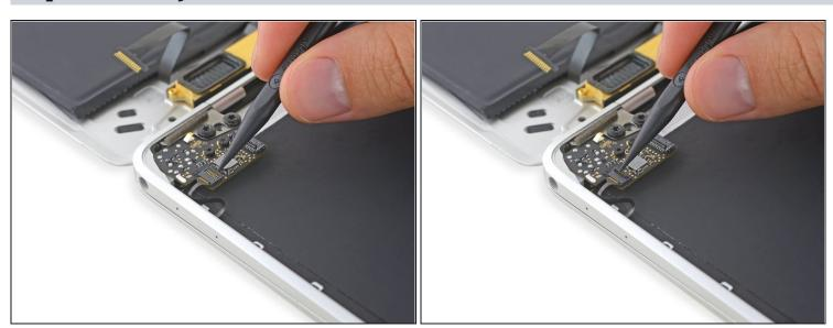
• Use a spudger to flip open the ZIF connector retaining flap for the dual microphone assembly ribbon cable.
