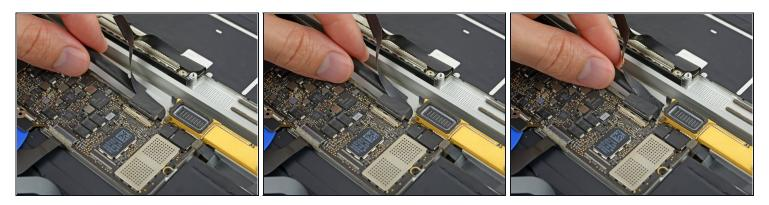
Carefully slide the flat end of a spudger underneath the display cable to separate the adhesive holding it to the lower case.
