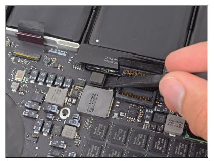
Use the flat end of a spudger to pry the trackpad ribbon cable connector up from its socket on the logic board.
