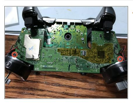
Remove the 2 Torx (T6) screws
