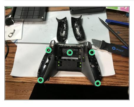
Remove the 5 Torx Security Bit (TR9) screws
