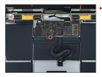
Remove the single 2.9 mm T5 Torx screw securing the battery connector to the logic board.
