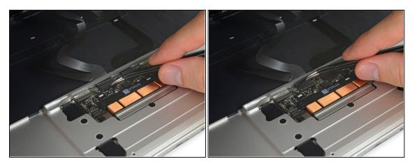
• Use tweezers to peel back the tape covering the trackpad cable ZIF connector.
