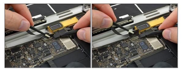
(i) It's possible the metal retaining flap on the display cable connector may flip open, remaining stuck to the tape.
