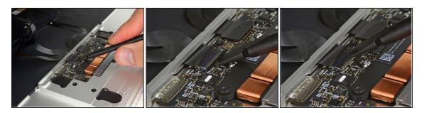
• Use a spudger to carefully flip up the retaining flap on the trackpad cable <u>ZIF connector</u>.
