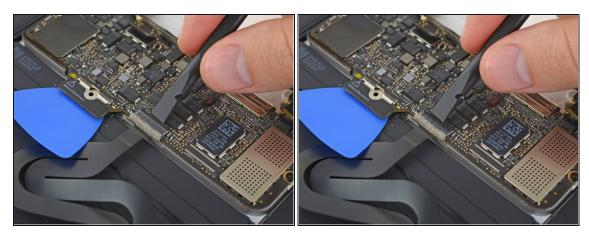
• Use a spudger to flip up the retaining flap on the trackpad cable ZIF connector.
