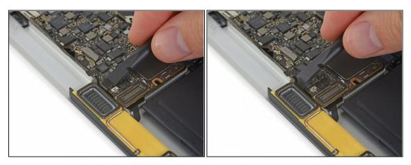
• Use a spudger to disconnect the left speaker cable connector by prying it straight up from the logic board.
