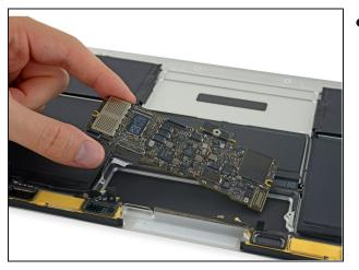
• Remove the logic board.
