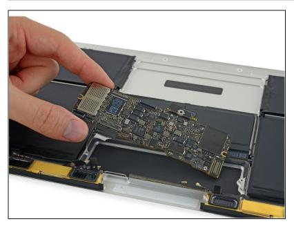
• Remove the logic board.
