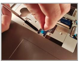
Locate the two flat cables and remove them carefully.
