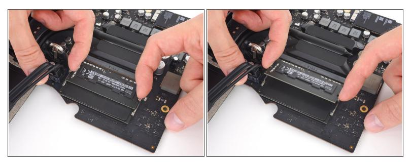
• Two clips secure the RAM module in place, one on each side. Using your fingers, spread the clips away from the RAM module.
